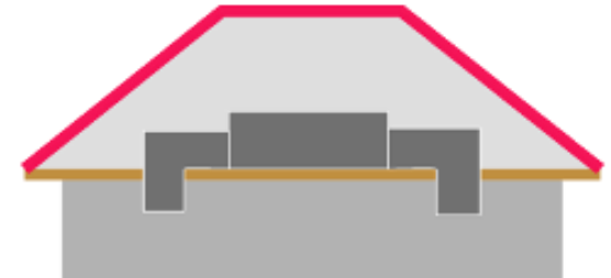
Ducts in Unvented Attic
